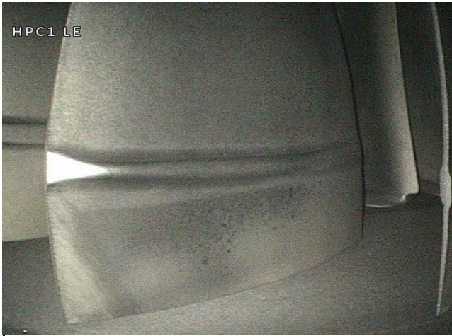
STAGE 1 HPC: SEVERAL HPC1 LE BLADES OBSERVED WITH MINOR DENTS TO LE IN LOWER 25%, DIM B & DIM A. ALL WITHIN AMM LIMITS. SEE DEFECTS PAGE FOR DETAILS
