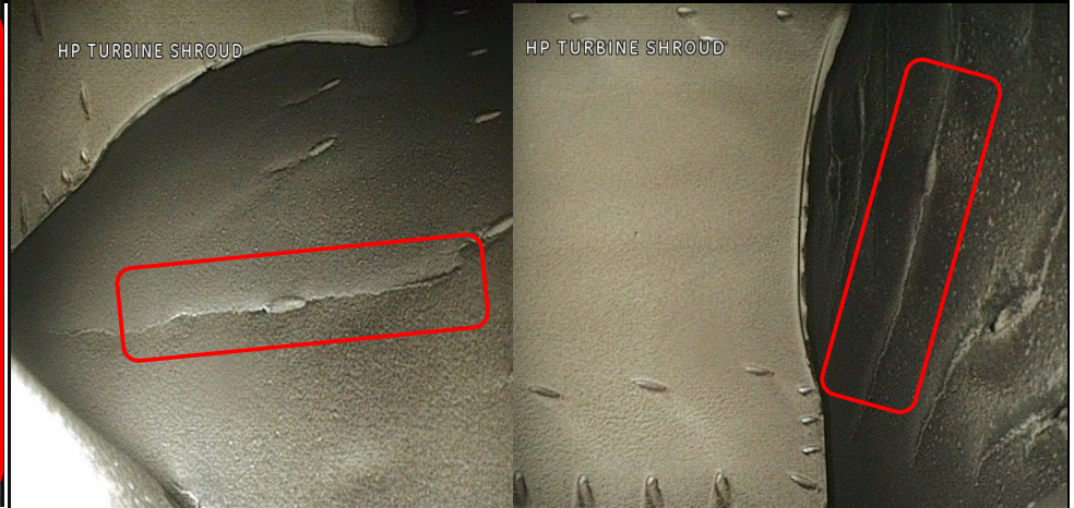
SEVERAL HPT SHROUD PANELS OBSERVED WITH AXIAL CRACKS STARTING FROM COOLING HOLES. ACCEPTABLE IN ANY AMOUNT AS PER AMM 72-00-00-200-815-F00.11.F.(1).(a).1) SERVICEABLE - NO LIMITATION. SEE APPENDIX M FOR CLARIFICATION.
