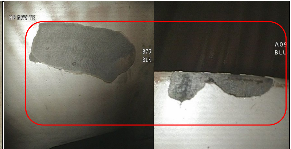
SEVERAL HPNGV TE OBSERVED WITH MISSING T.B.C TO BOTH CONCAVE AND CONVEX SURFACES.ACCEPTABLE IN ANY AMOUNTS AS PER 72-00-00-220-801-F00.8.G.2.(d).1) & (3).(c).1). SERVICEABLE- NO LIMITATION.
