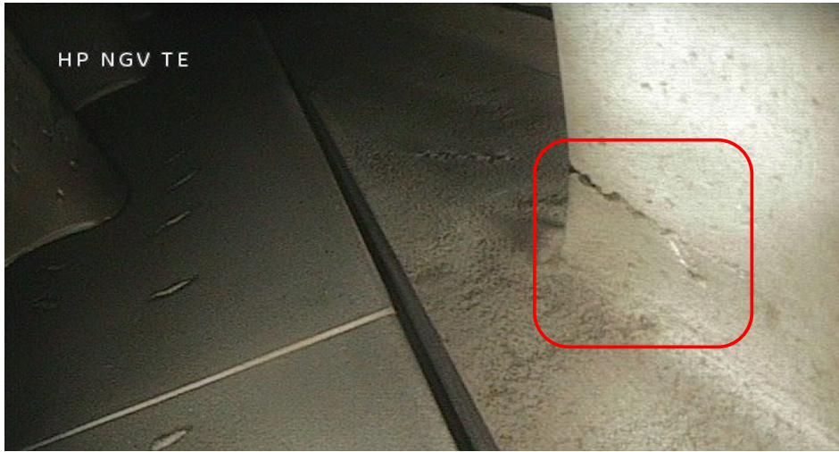
SEVERAL HPNGV TE OBSERVED WITH CRACKING TO TE. CRACKS.ACCEPTABLE IN ANY AMOUNTS AS PER 72-00-00-220-801-F00.8.G.(4).(a).1). SERVICEABLE- NO LIMITATION. SEE APPENDIX K FOR CLARIFICATION.
