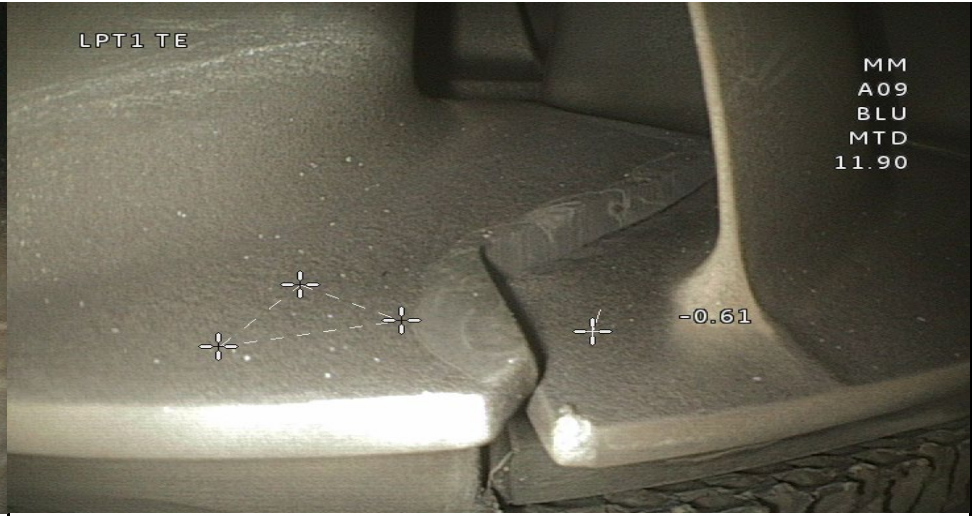
LPT 1 BLADES OBSERVED WITH OUT OF FLUSH IN THE TE TIP SHROUD INTERLOCK. OUT OF FLUSH MEASURED AT - 0.61MM. WITHIN AMM 72-00-00-200-808-F00.12.G.(2).(j).1.(a) THAT INTERLOCK FACES ARE NO MORE THAN 1.20MM OIUT OF FLUSH. SEE APPENDIX O FOR CLARIFICATION.
