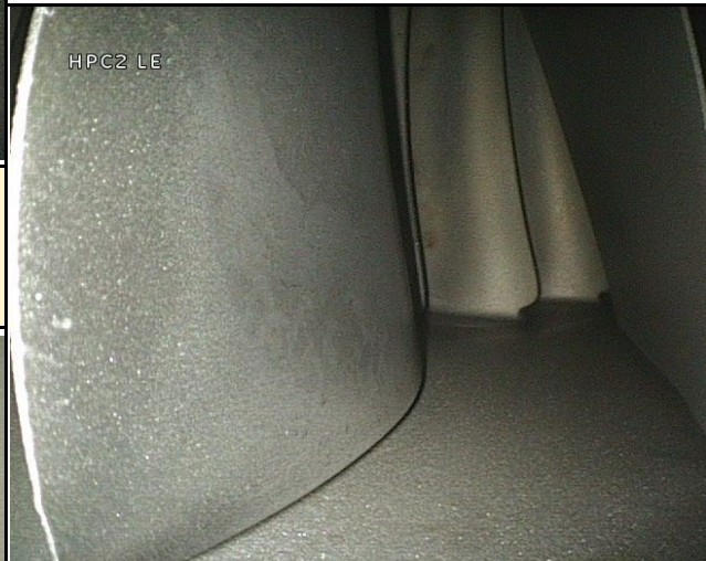
STAGE 2 HPC: SEVERAL HPC2 LE BLADES OBSERVED WITH MINOR DENTS TO LE IN LOWER 25%, DIM B & DIM A. ALL WITHIN AMM LIMITS. SEE DEFECTS PAGE FOR DETAILS. 1 OFF HPC2 BLADE OBSERVED WITH LE DENT IN AMM LIMITS
